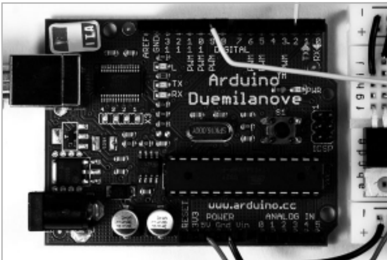
FIGURE 6-29 Powering a breadboard with the Arduino
