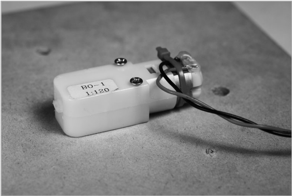
FIGURE 10-6 Motor mounted on the underside of the box top
