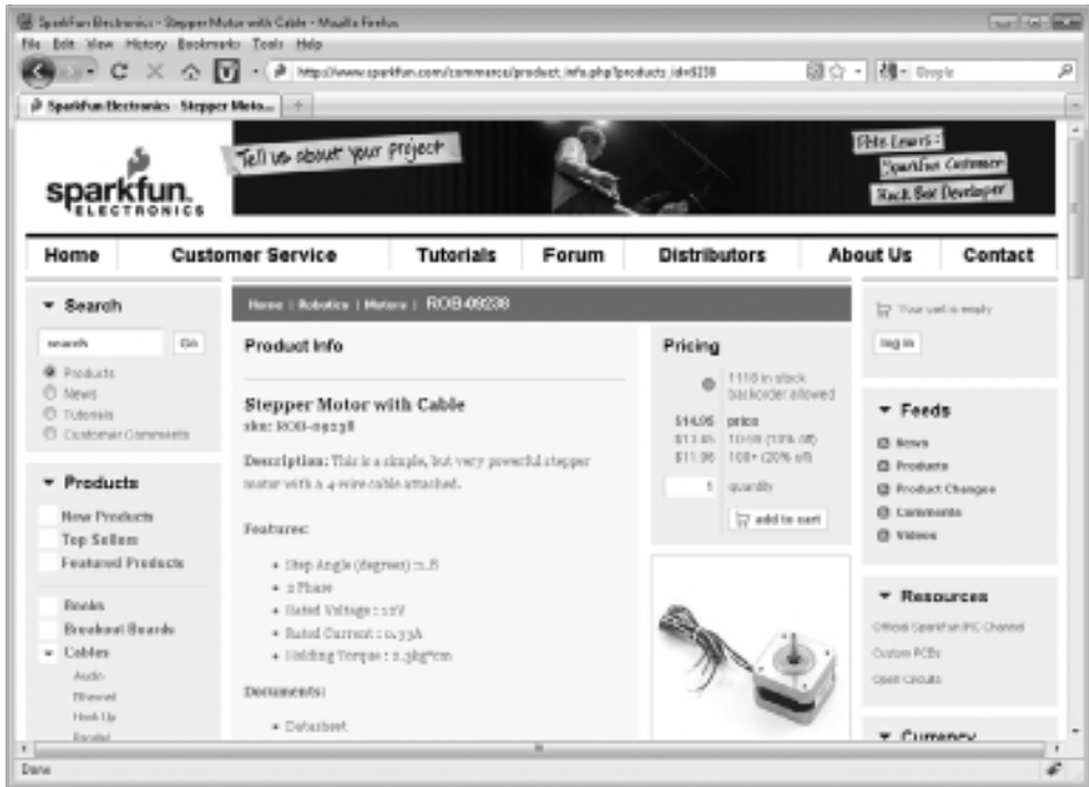
FIGURE 6-11 Features of SparkFun's ROB-09238 stepper motor
