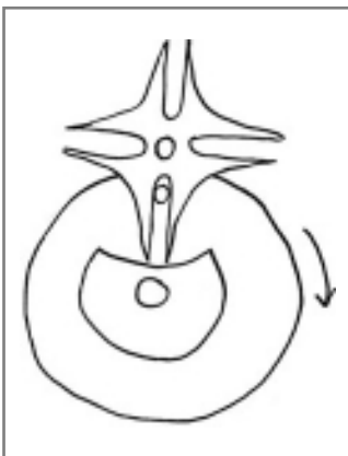
FIGURE 8-12 A Geneva stop mechanism
