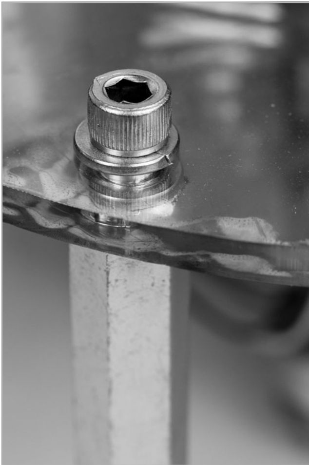
FIGURE 10-12 Detail of installing the standoffs
