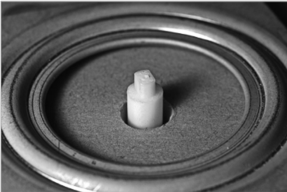
FIGURE 10-4 Shaft adaptor centered in the box top
