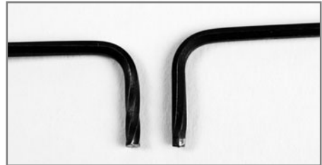
FIGURE 2-2 Allen keys that failed in torsion
