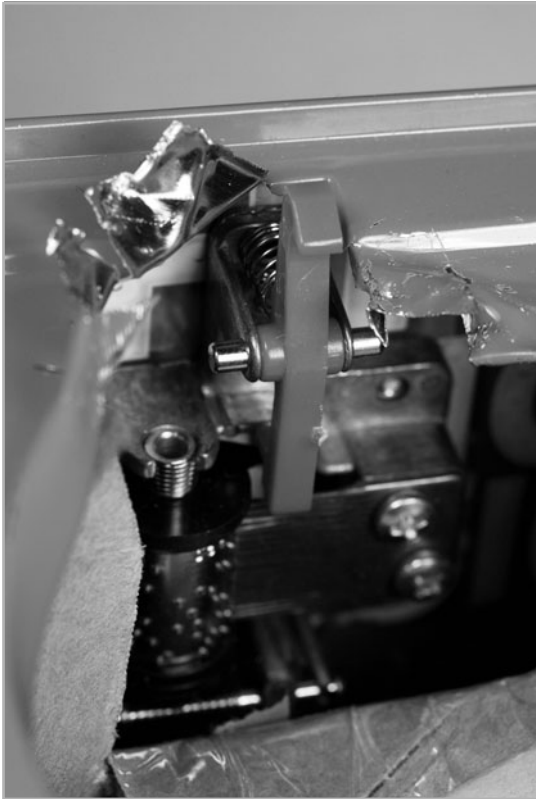
FIGURE 7-44 A compression spring returns the latch in a jack-in-the-box.
