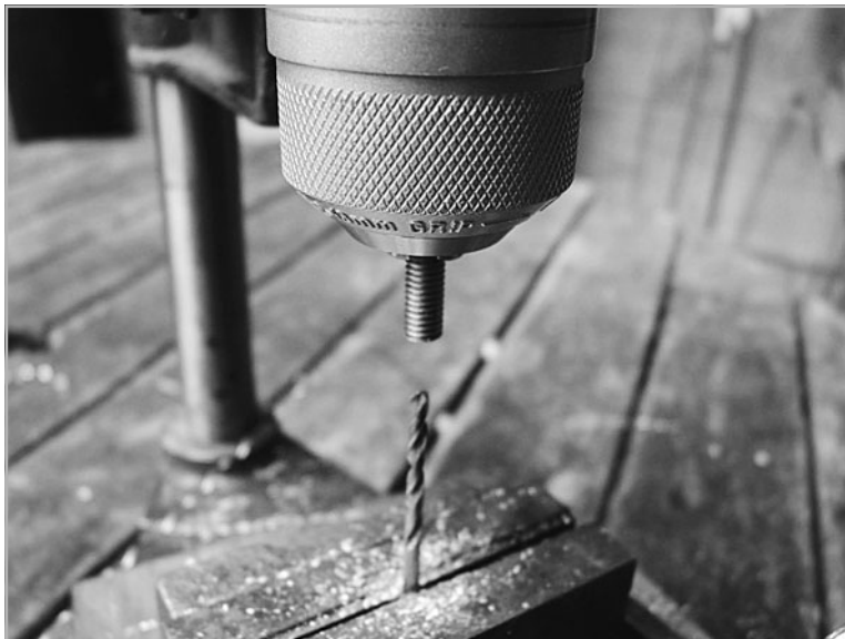
FIGURE 9-6 Part in drill chuck ready to go (credit: Vik Olliver)
