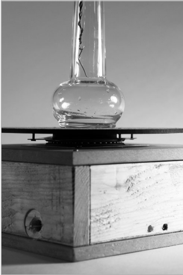
FIGURE 10-7 Rotating tabletop mounted on box top
