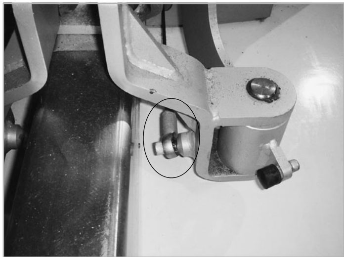
FIGURE 7-11 Spherical bearings are used on gym equipment to accommodate misalignment in the cable pull direction.
