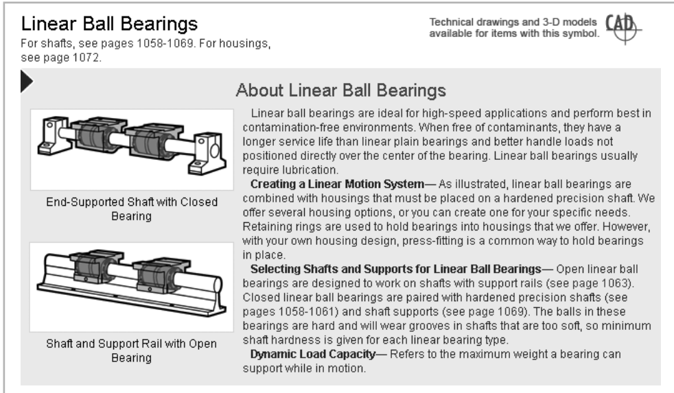
FIGURE 7-8 Linear ball bearing configurations (credit: McMaster-Carr)
