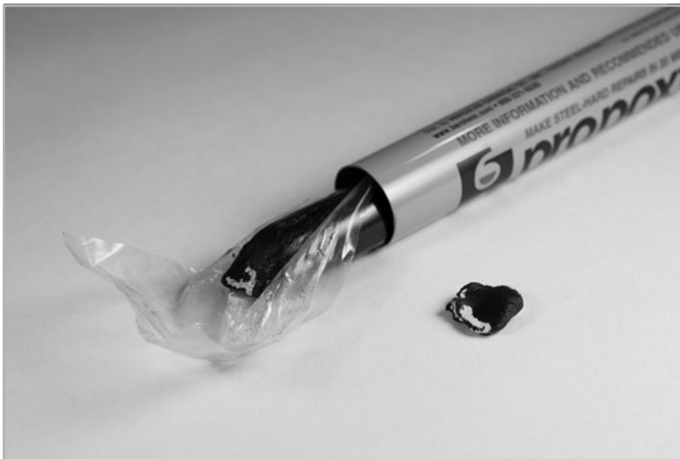
FIGURE 3-11 Epoxy putty—the great project saver
